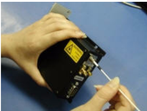
Figure 22 Cleaning the Optical Port [2]
